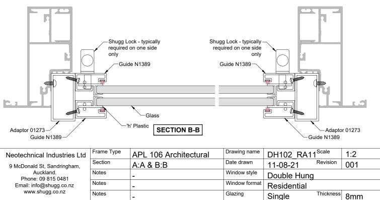
Details subject to change without notice. Exterior frames by others, Neotechnical Industries Ltd does not own the rights to exterior frames shown and are indicative only. All other details © Neotechnical Industries Ltd, not to be reproduced, altered or distributed in any form without permission.
